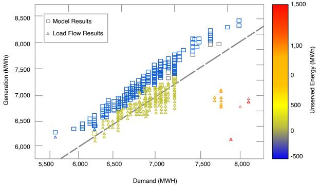
Note: The graph shows the model results alongside load flow results at the close-call margin of 500 megawatt hours (MWh). The results below the dashed line constitute shortfalls. The color of each datapoint is based on the difference between generation and demand at that point.
